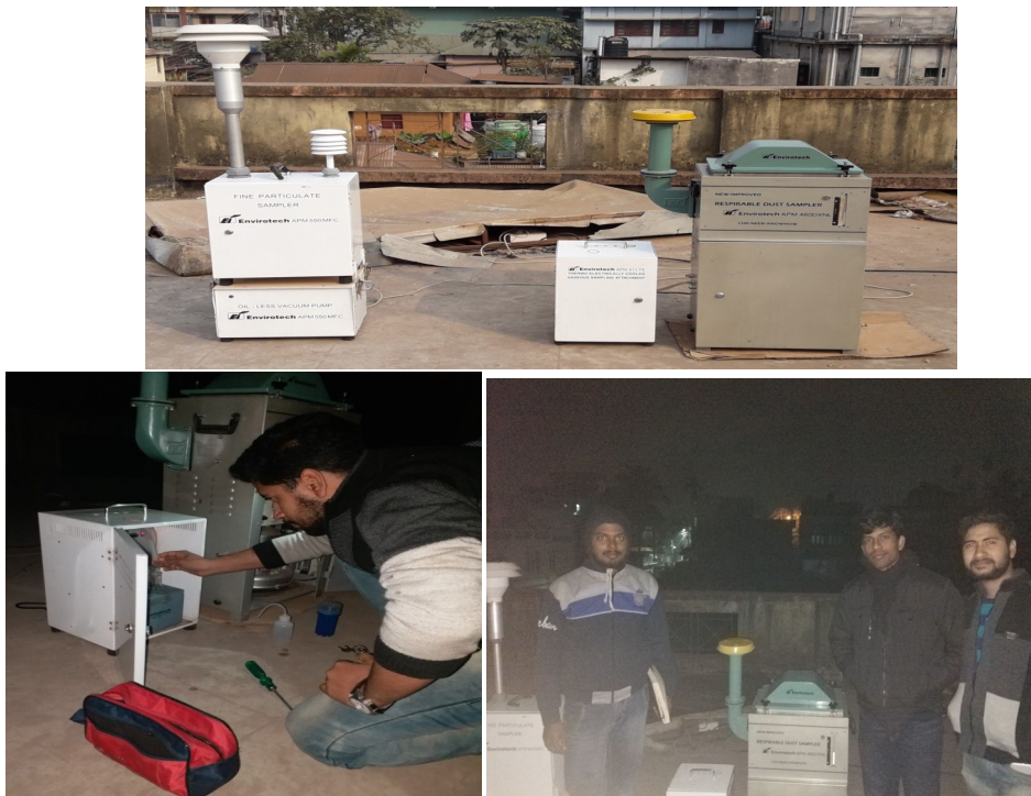
Figure 5: Respirable dust sampler for PM_{10} and Fine particle sampler for PM_{2.5}
