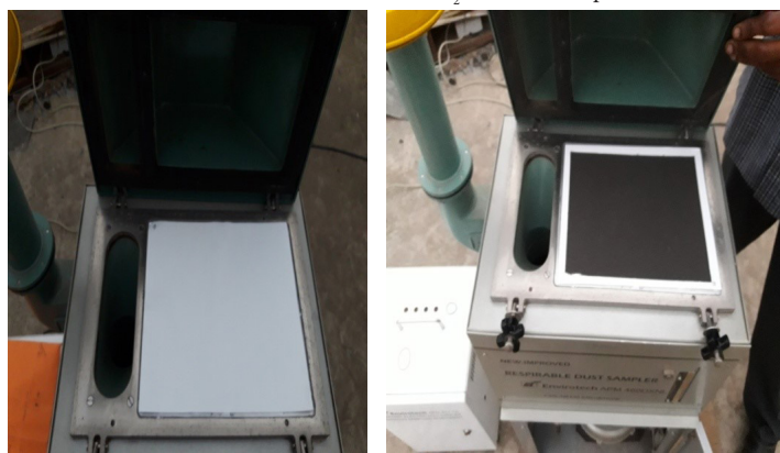
Figure 6: Before and after experiment of \text{PM}_{10} sampling filter paper
