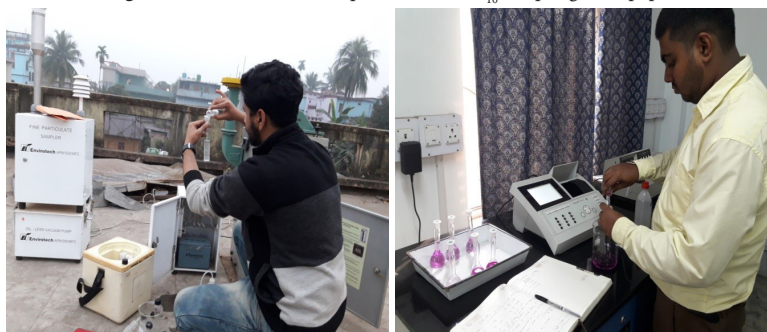
Figure 7: Measuring the value of \text{SO}_x and \text{NO}_x
